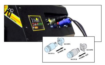
It is recommended to Daisy Chain a Max of 10 fixtures, even if the limitations imposed by DMX Standards are for an higher q.ty of units and even if the Powercon Connections are rated for 20A max.
