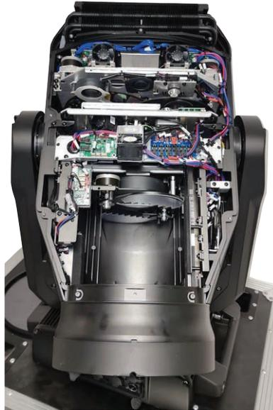
2. Unplug the power and data cable for the module, then remove the four (4) module screws holding the module in place, as indicated by the arrows in the image below. Pull the module gently towards you, taking care to ensure that the module does not catch or snag on any surrounding cables.
